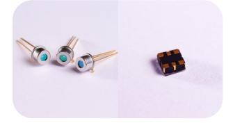
*Noiseless InGaAs*<sup>®</sup> refers to Phlux's patented compound semiconductor technology, which enables APDs to operate exceeding avalanche gain of 100 without excess noise factor induced degradation of the signal-to-noise ratio (SNR).
