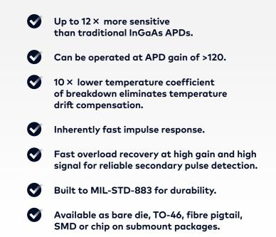
Note: The term Noiseless InGaAs™ is used to describe Phlux's patented compound semiconductor technology that is used to manufacture APDs with an excess noise factor low enough to enable an APD gain of over 100 without SNR deterioration.
